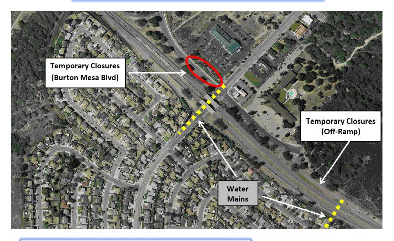
This July, VVCSD is contracting with SAK Construction, LLC to reline two 12" water mains under Hwy 1. These critical pipelines, providing water to south village, are over 50 years old and require rehabilitation to repair leaks and extend their life.
